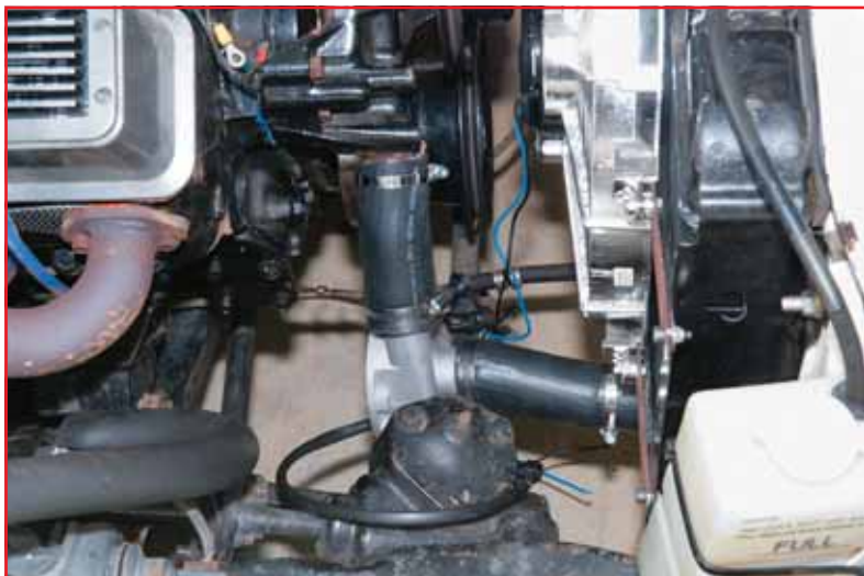
The pump sits neatly in the vacant spot under the water pump and clears the sway bar underneath too.
