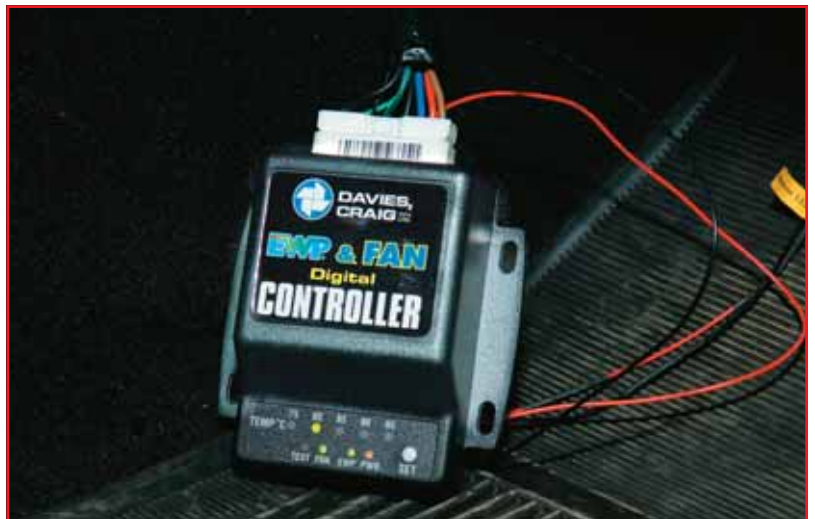
The lights on the controller show that the engine is at 80°C, the unit has power, the electric water pump is on and the Thermatic fan is on.
