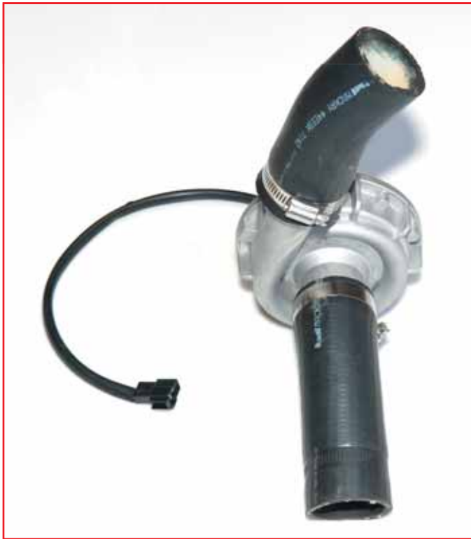
The electric water pump has been grafted into the Chev's bottom radiator hose.
