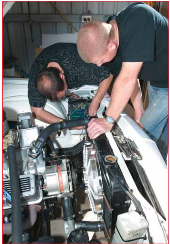
Wiring the relay for the Thematic fan was the final job.
