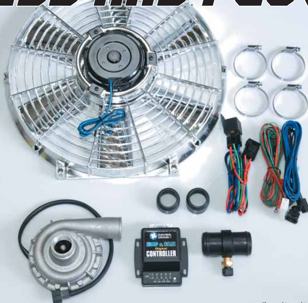
The two kits combined include the electric water pump, a Thermatic fan, a digital controller and all the hardware needed for installation.
