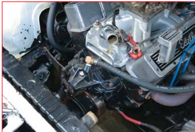
The fan and shroud are removed to reveal the stock water pump.
