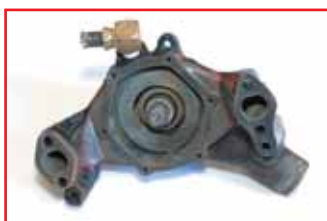
The stock impeller with the fan blades removed.
