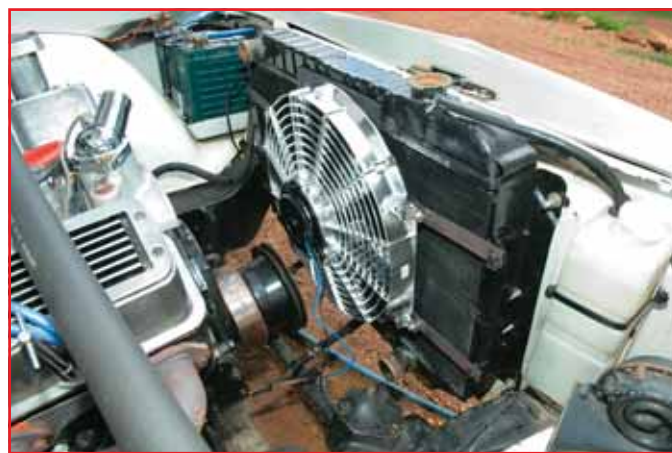
The 16-inch Thematic fan is bolted into place.
