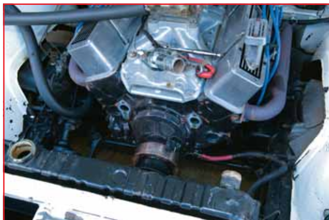
The water pump is removed for some minor surgery.
