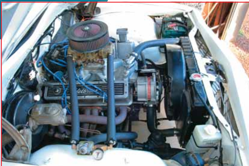
The 400 Chev was originally cooled by a conventional water pump and a clutch fan.
