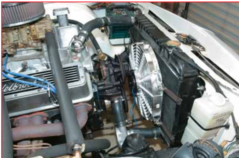
The modified water pump has been re-installed and the system filled up with coolant. The system now needs to be wired.
