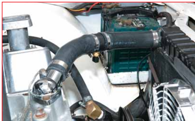
A temperature sensor for the digital controller is mounted in the top radiator hose.
